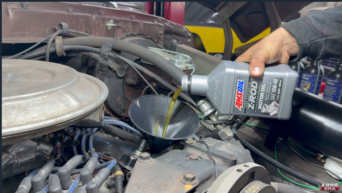
The fill: Z-ROD 10W-40 poured through the funnel at the pre-trip build. Survive Route 66, 21:11.
